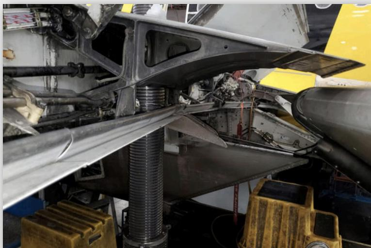
Whilst being held up on jacks, [it appears that the aircraft slipped off, or a jack moved from its position](#), resulting in serious damage to the airframe. Pictures of the accident show the jacks penetrating the fuselage and wings:
