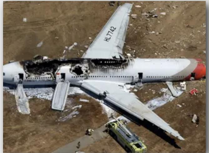
But the board also said the complexity of the Boeing 777’s auto-throttle and auto flight director — two of the plane’s key systems for controlling flight — **contributed to the accident**. Materials provided to airlines by Boeing that **fail to make clear** under what conditions the auto-throttle doesn’t automatically maintain speed were also faulted.
